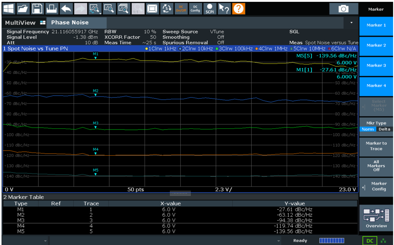
Figure 36: Spot noise vs tune PM measurement result
