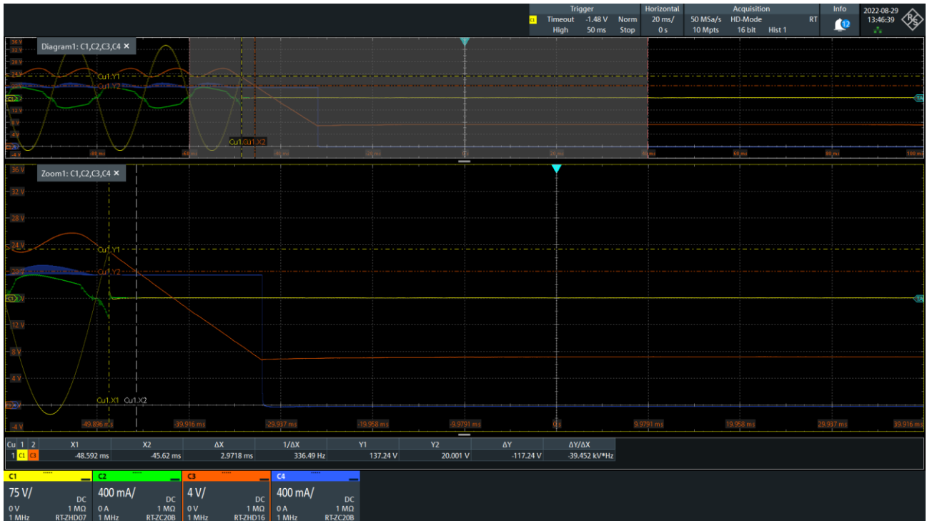
Figure 32 Turn-off Delays with AC Mains Input
