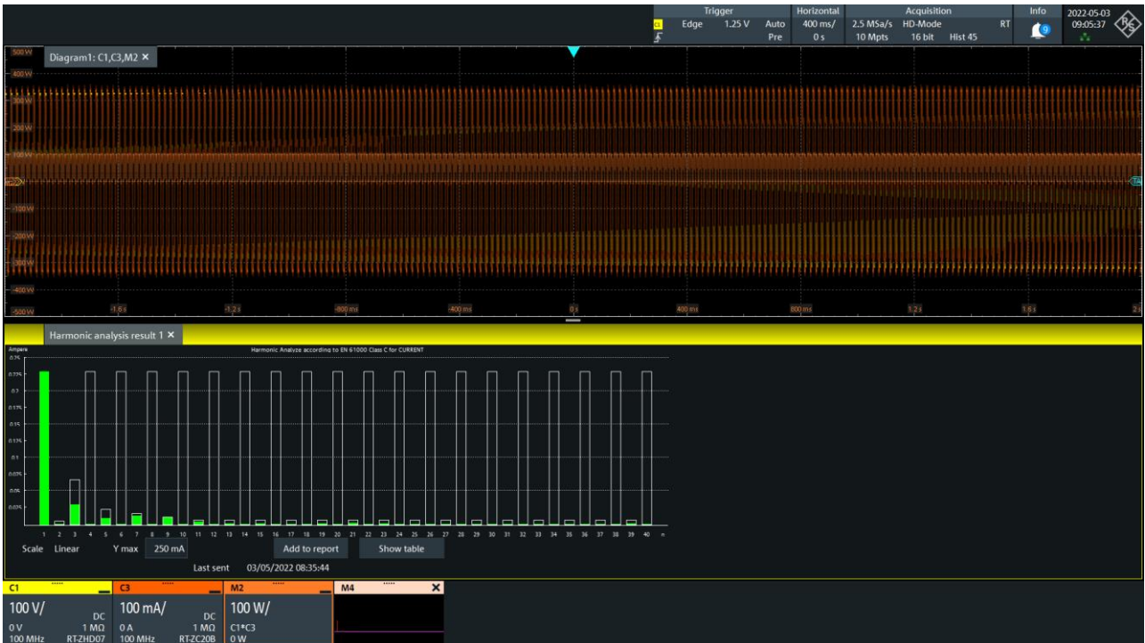
Figure 13 Current Harmonic Measurement Bar View
