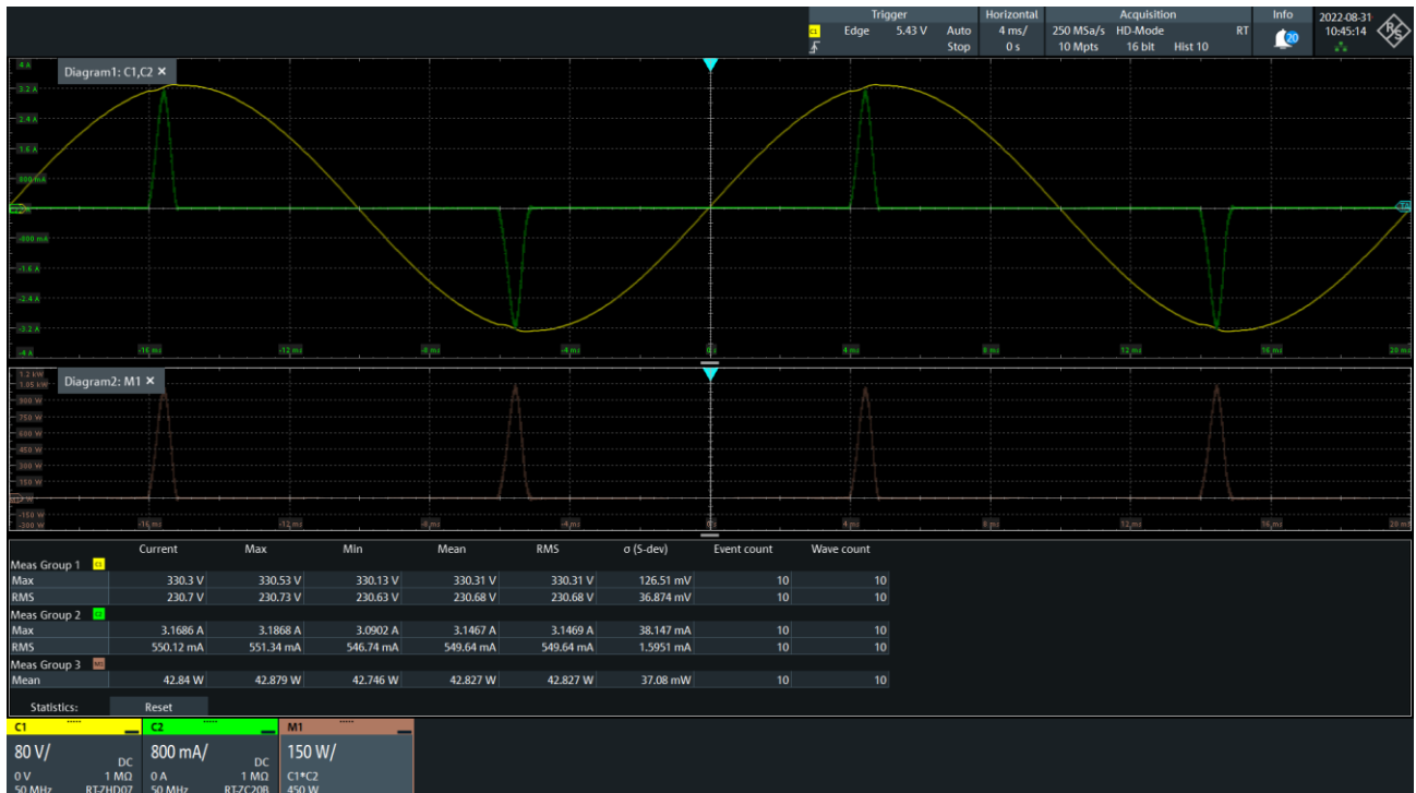
Figure 10 Measured Voltage, Current and Power at Input Terminals (Non-PFC)
