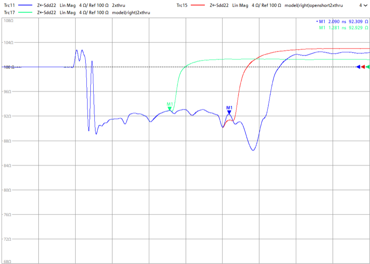
Figure 19 TDR plot comparing the right-side models
