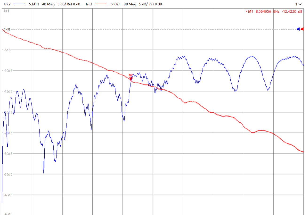
Figure 7 return loss (blue) and insertion loss (red) of balanced S-parameters of the 2xthru measurement. (2 GHz/div)
