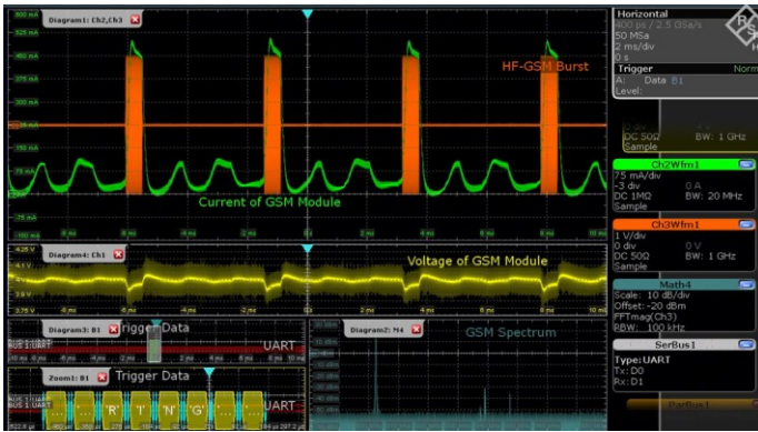
Figure 3-9 An example of multi-domain analysis on R&S®RTP
