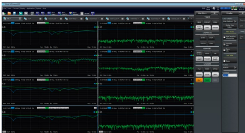
Figure 3-12 Characterization of a beamformer IC using multiport VNA R&S®ZNBT
