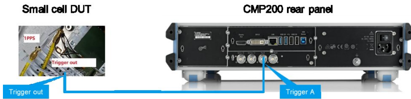
Figure 2-19 Cabling of trigger signal between small cell DUT and CMP200
