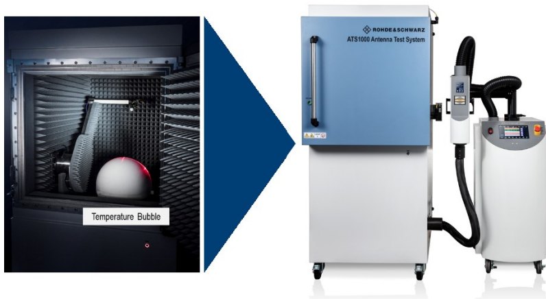
Figure 3-15 R&S®ATS1000 with temperature bubble
