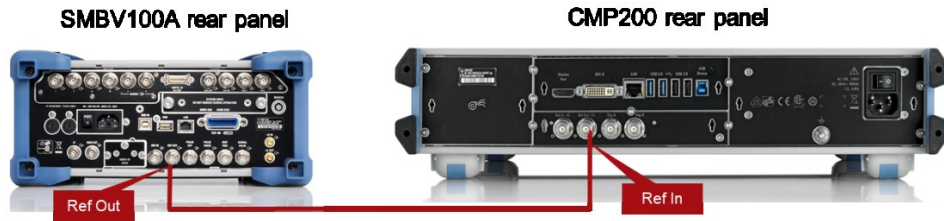
Figure 2-15 Cabling of 10 MHz reference between R&S®SMBV100A and CMP200
