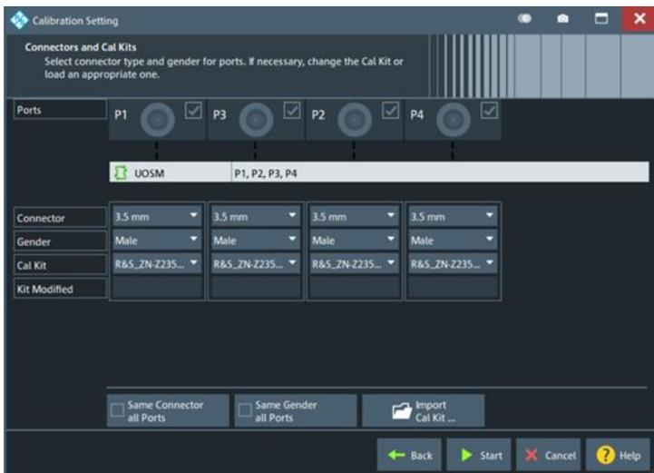
5. Start calibration and connect all required calibration standards (open, short, match and unknown through).
