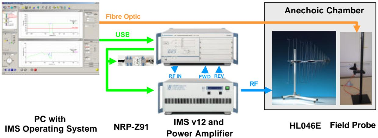
The block diagram shows the general setup of a test system according IEC / EN 61000-4-3. It covers radiated fields in the frequency range 80 MHz to 2 GHz. The field strength in 3 m test distance and over an area of 1,5 x 1,5 m is 10 V/m. This configuration for 10 V/m is used by most customers.
