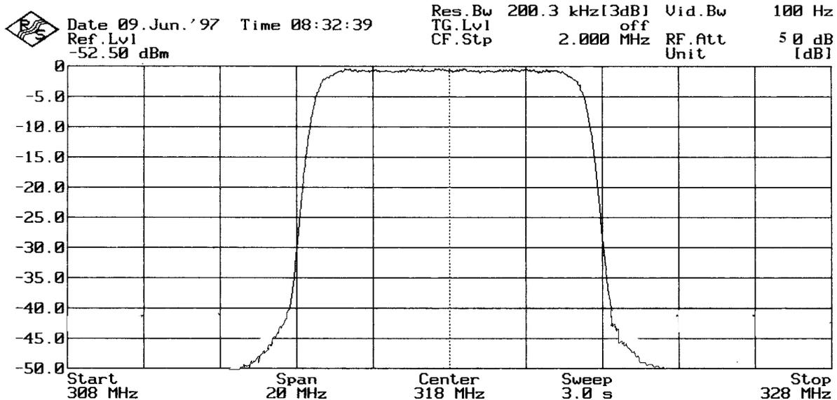
Power distribution in an 8-MHz channel with 64QAM modulation
