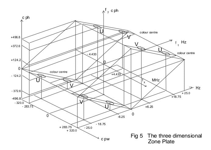
The diagram shows that the colour centres change at a rate of  $\pm$  18.75 Hz at  $\pm$  124 lines about the centre of the picture, while the coloured circles just about visible at the upper and lower margins of the picture change at a rate of  $\pm$  6.25 Hz.
