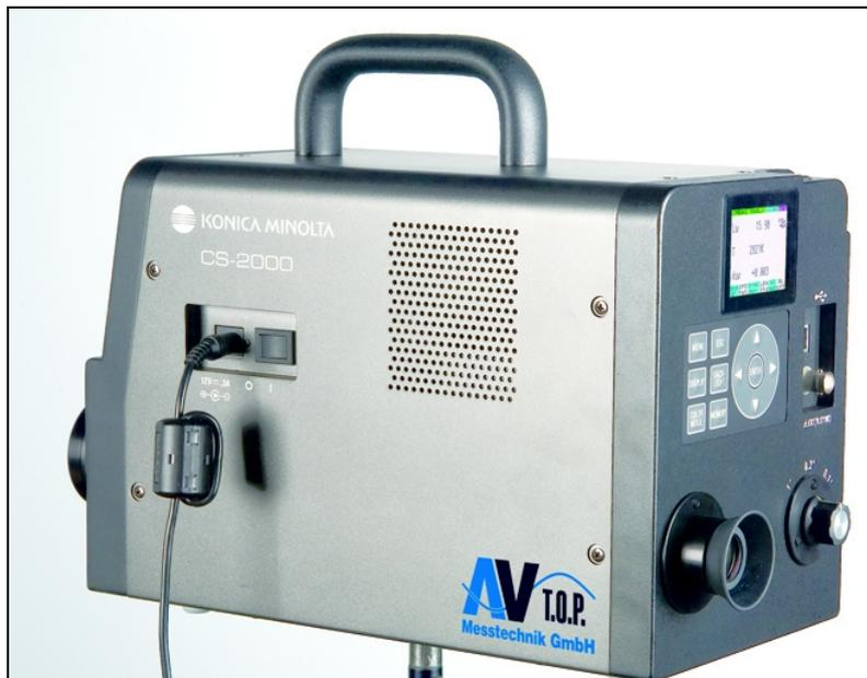
Figure 3: Konica Minolta CS-2000 spectroradiometer
