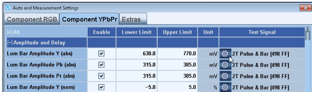
Fig. 6-7: Opening the dialog box for setting the test signal, test line position and test point positions.
