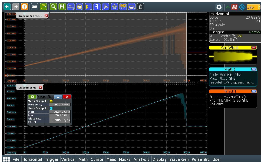
Fig. 2-15: Diagram1 (blue trace) shows the low pass filtered demodulated chirp signal in time domain beginning at 77 GHz
