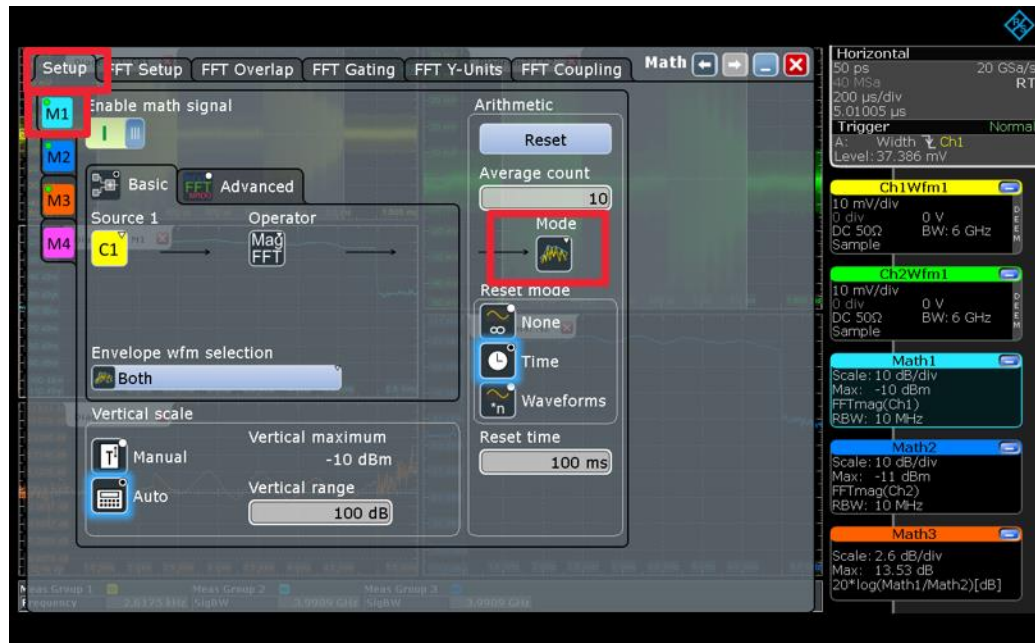
Fig. 3-3: Setup Math Signal M1
