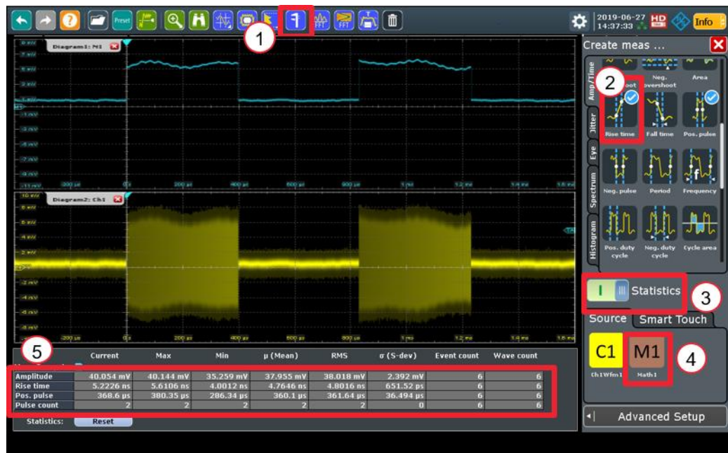
Fig 2-10: Measurement settings and results for certain pulse envelope parameters
