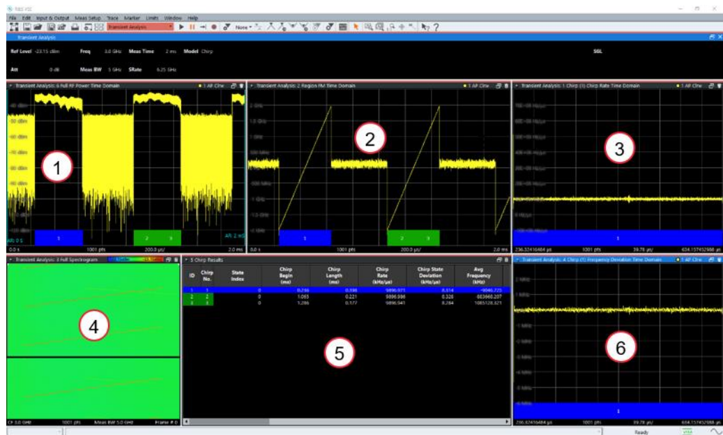
Fig. 2-20: Chirp analysis with the VSE software
