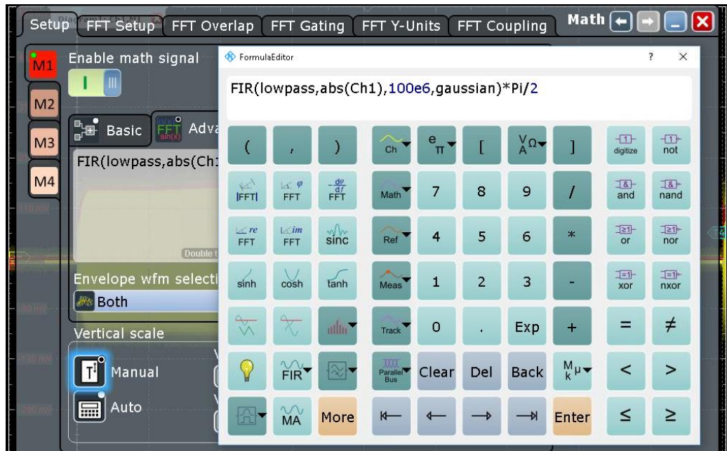
Fig. 2-8: This low pass filter formula removes the RF carrier and creates the pulse envelope
