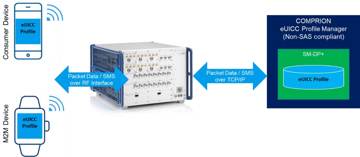
Fig. 2-2 eUICC test solution for non-SAS compliant M2M and consumer device with R&S® CMX and COMPRION® eUICC Profile Manager
