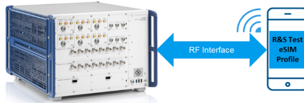
Fig. 2-3 eUICC test solution for SAS compliant consumer device with R&S® CMX and COMPRION® eSIM Test Profile Service
