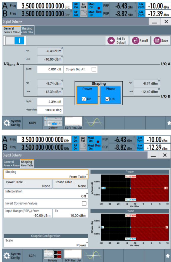
Fig. 5-1: Two GUI screens of the SMW-K546 software, (i) the "General" tab, with overview of the splitting and (ii) the "Shaping" tab, with its control of the Doherty auxiliary path characteristics.
