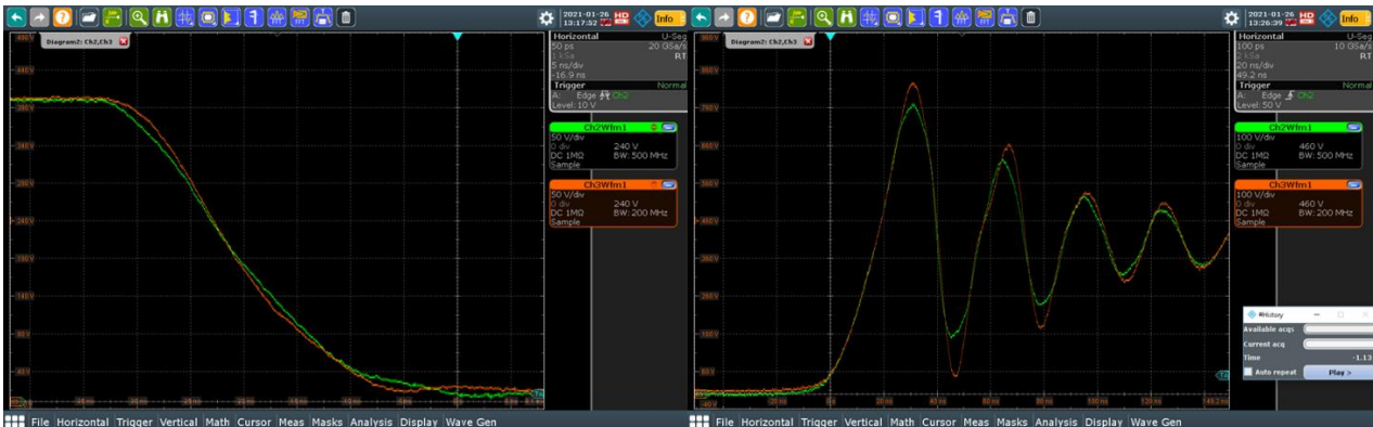
Figure 29: Turn-on (left) and turn-off (right) measurements of v_{DS} with different probes
