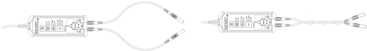
Figure 17: Ways to use differential probes. Using twisted leads provides usually the best measurement result as unintended noise coupling is minimized.
