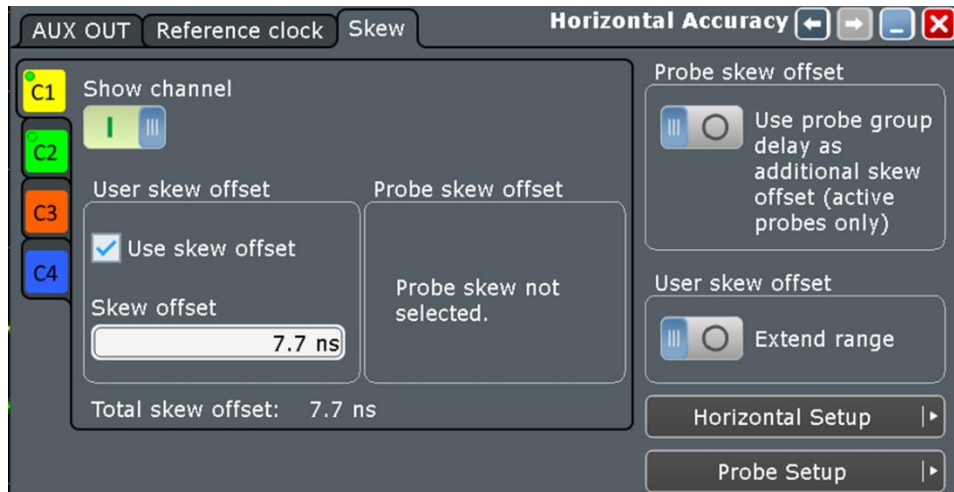
Figure 35: Correcting the time offset with the integrated de-skew function of the oscilloscope.
