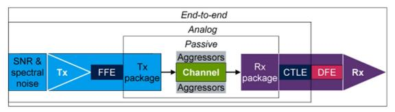
Figure 17: Separating the elements of an IBIS-AMI simulation.
