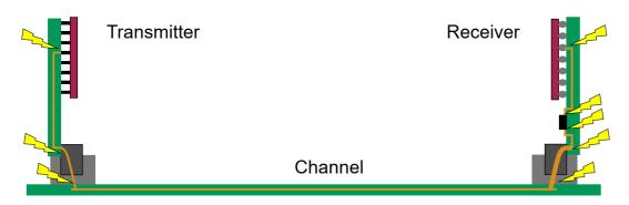
Figure 15: Long reach configuration with multiple discontinuities and corresponding reflections.
