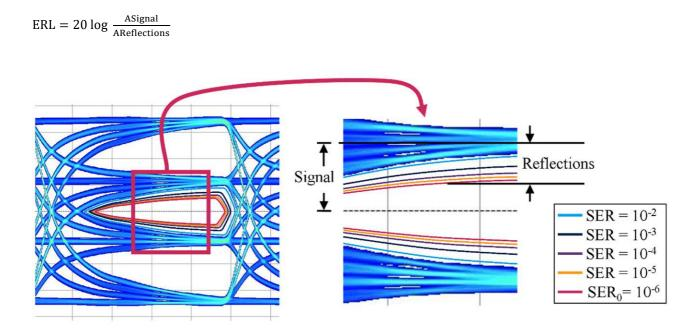
Figure 16: Like COM, also ERL is an SNR-like figure of merit, calculated from the measured S-parameters based on a defined model of the overall transmission system.
