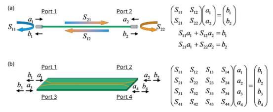
Figure 5: S-parameters: (a) 2×2 S-parameter matrix for a single trace or cable and (b) 4×4 S-parameter matrix for two channels.
