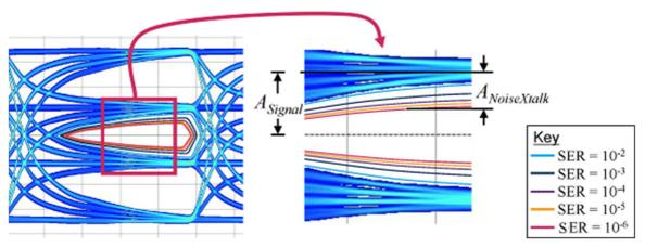
Figure 14: COM is an SNR-like parameter calculated from an eye diagram derived from the pulse response of a system model that is defined by the channel S-parameters.
