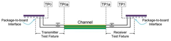
Figure 9: The channel model and test points.
