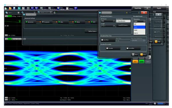
Figure 12: PAM-4 eye diagram calculation.
