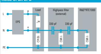
Fig. 2: Test setup to measure the common mode noise of an EPS
