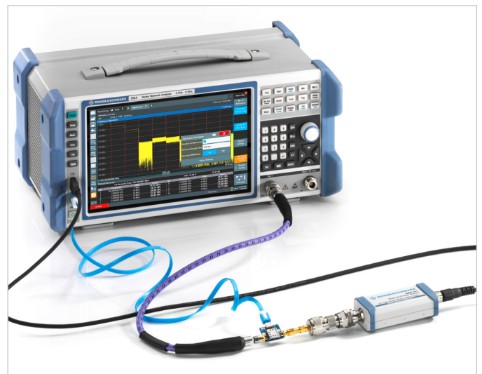
The power sensor NRP18T supports measurements from -35 dBm to +20 dBm from DC to 18 GHz.
