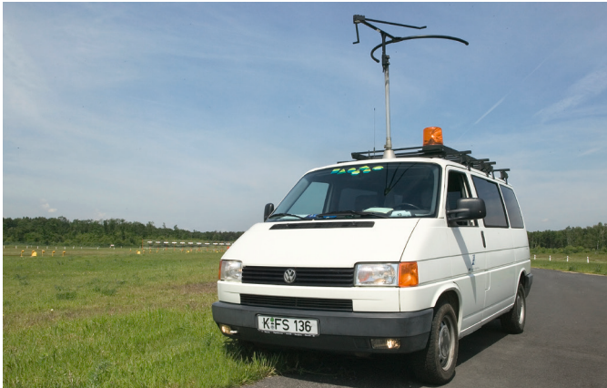
Measurement vehicle for verifying ILS stations.
