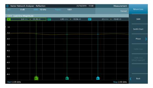
By manual calculation or the simple press of a button, the return loss is approx. 12 dB.
