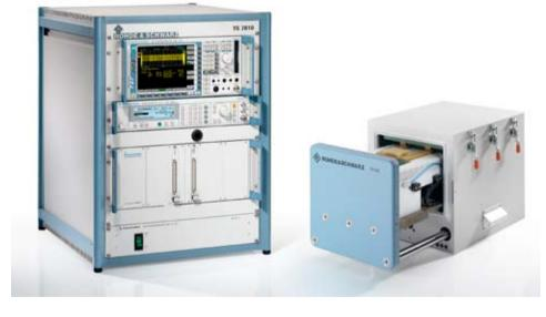
The RF Test System R&S®TS 7810 was designed specifically for automatically checking tire pressure sensors. It consists of a hydraulic test fixture with a pressure-proof chamber for holding the DUT and a 19" rack containing RF test instruments as well as the Open Test Platform R&S<sup>®</sup>CompactTSVP. You can easily add auxiliary components such as an RF generator to the system. This may be necessary, for example, when you need to test the counterpart of the pressure sensor, the receiver chip.
