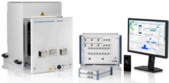
$R\&S^{\circ}CMX500~5G$  radio communication tester: FR1/FR2 test setup for data throughput testing.
