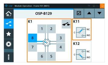
The R&S<sup>®</sup>OSP instruments can be controlled and configured via Ethernet using the web GUI or SCPI commands. Alternatively, they can be controlled via the GPIB-to-LAN converter using SCPI commands.
