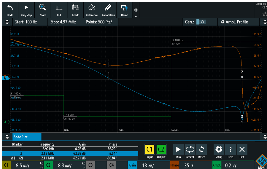
Measurement of the stability of a DC/DC converter (blue trace: gain; orange trace: phase; green trace: amplitude profiling of the stimulus signal)
