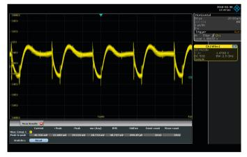
Measurement of a 1.5 V power rail using an R&S®RT-ZPR20 1:1 active power rail probe (–38.3 mV (V<sub>pp</sub>)). The captured waveform includes higher frequency transients riding on the rail.
