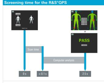
After stepping onto the scanner's footprints and slightly raising your arms away from your side as shown on the panel, the operator presses the scan button. The screening process seems nearly instantaneous to both the passenger and operator.
