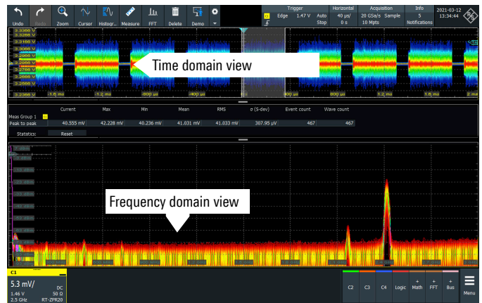
Frequency domain views of power rails to find coupled sources that are impossible to see in the time domain.
