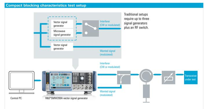
Providing the wanted and interferer signals up to 20 GHz and high output power in one box makes the two-path R&S\*SMW200A an efficient solution for blocking characteristics tests.
