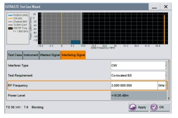
Standard-compliant blocking conformance tests for LTE and WCDMA base stations can be remarkably simplified by test case wizards, which are an integral part of the related digital standard software option. The wizards automatically configure all wanted and interfering signal parameters and provide a graphical overview of the generated test signals.
