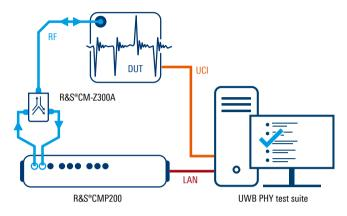
The UWB PHY test suite, which is based on the industryproven R&S®WMT test automation framework, allows fully automated execution of the FiRa<sup>™</sup> test cases as required by authorized test laboratories for FiRa<sup>™</sup> certification. At the end of a test run, the tool provides an overall pass/fail verdict and all details about the performed tests. Finally, it generates a tamper-proof test report containing all relevant information required to apply for FiRa<sup>™</sup> certification.
