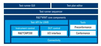
The UWB PHY test suite is especially beneficial for R&D engineers to perform preconformance testing. This solution provides the expected flexibility via an easy-to-use graphical user interface (GUI).
