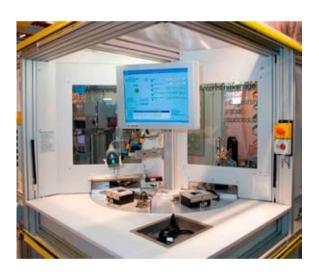
The implementation of the system described here is based on a rotary table with integrated automatic functional testing. The system not only performs the electrical functional tests in the DC and RF range. It also fastens the electronic module on the base with the housing parts while applying torque control to the screws. Mechanical and visual aspects of the housing and of the various mounting screws are checked during the production process by means of a camera system.
