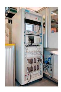
The test system also controls the rotary table and manages and monitors all electrical and mechanical parameters. Every step of production from the setup of the individual jobs to the management of the transport containers is monitored and documented. A sensor-controlled gate detects and labels defective (FAIL) parts and separates them from the good (PASS) parts. The result is minimum cycle time at maximum process stability.
