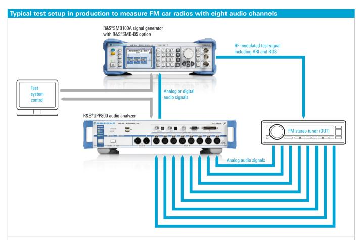
The R&S®UPP800 audio analyzer generates all required audio test signals and transfers them to the R&S®SMB100A, which adds the ARI and RDS test signals and modulates the whole test signal onto the RF carrier. The DUT demodulates the received test signal and outputs the audio signals in all amplifier channels. Measuring these signals with the R&S®UPP800 closes the loop and makes it possible to analyze the overall sound quality of the car radio DUT.
