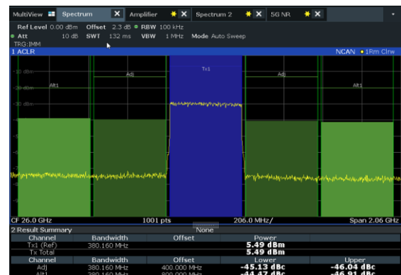
Figure 6 – ACPR performance at Reference input power
