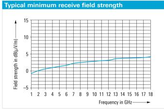
With R&S $^{\circ}$ HL024S9 (for a receiver with F = 15 dB,  $\Delta$ f = 1 MHz).
