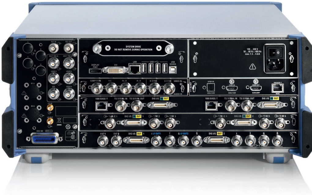
Rear view of the R&S®BTC with I/Q interfaces.
