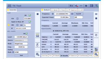
R&S°CMA180: The VoIP audio generator provides the IP connection and the audio input to the radio. The radio will modulate the digital audio signal and transmit it to the R&S°CMA180 over the air interface. The R&S°CMA180 then measures the RF parameters and the signal quality.
