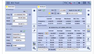
R&S\*CMA180: An AM signal with a 1020 Hz audio tone is provided to the DUT and the demodulated audio is measured on the VoIP interface.
