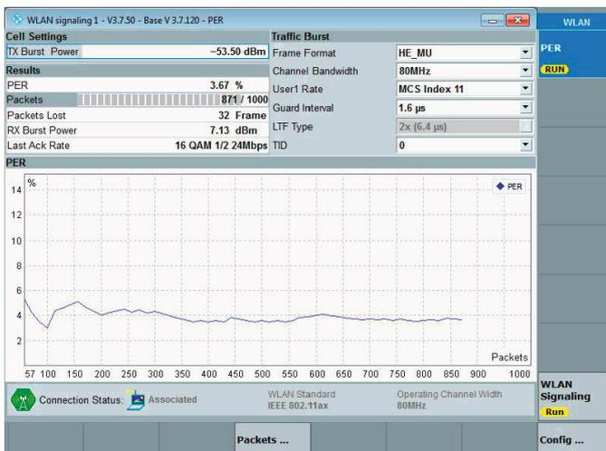
Automated RX performance test procedures with R&S<sup>®</sup>CMWrun.
