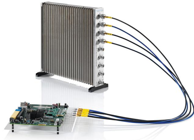
Test setup for the switched MIMO TX measurement. Each antenna in the DUT is connected to a port on one R&S®CMW100. The ports are switched in rapid succession to the test set's analyzer.
