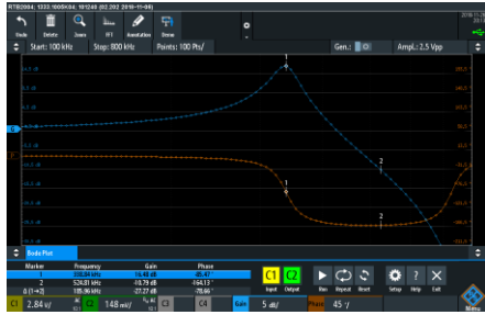
R&S®RTx-K36 frequency response analysis (Bode plot) options support R&S®RTB2000, R&S®RTM3000 and R&S®RTA4000 oscilloscopes
