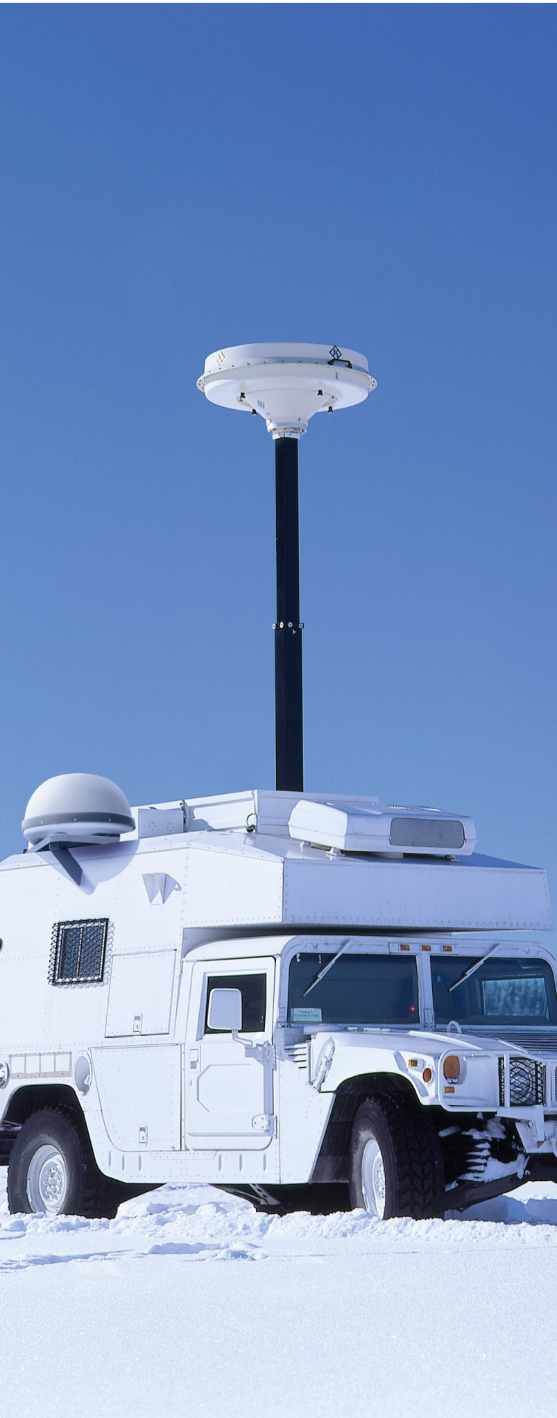
Mobile DF system with the R&S®DDF550 and the R&S®ADD253.
