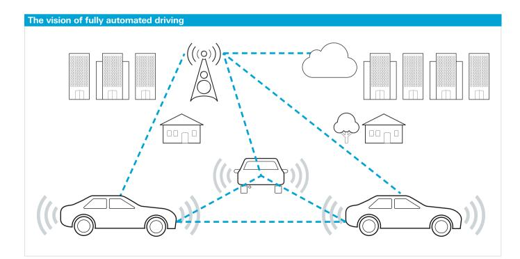
under discussion for managing such situations. In this case, a remote driver is connected to the vehicle via the cellular system. He steers the car based on camera images that are captured and transmitted with only a very brief delay. Technical challenges and legal frameworks make large-scale commercial implementation a mid- to long-term goal.
