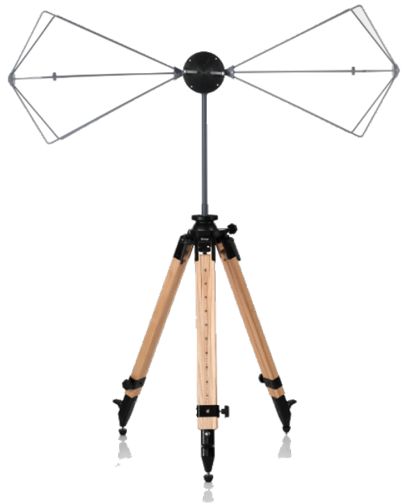
Figure 15 - Biconical antenna used in EMI testing
