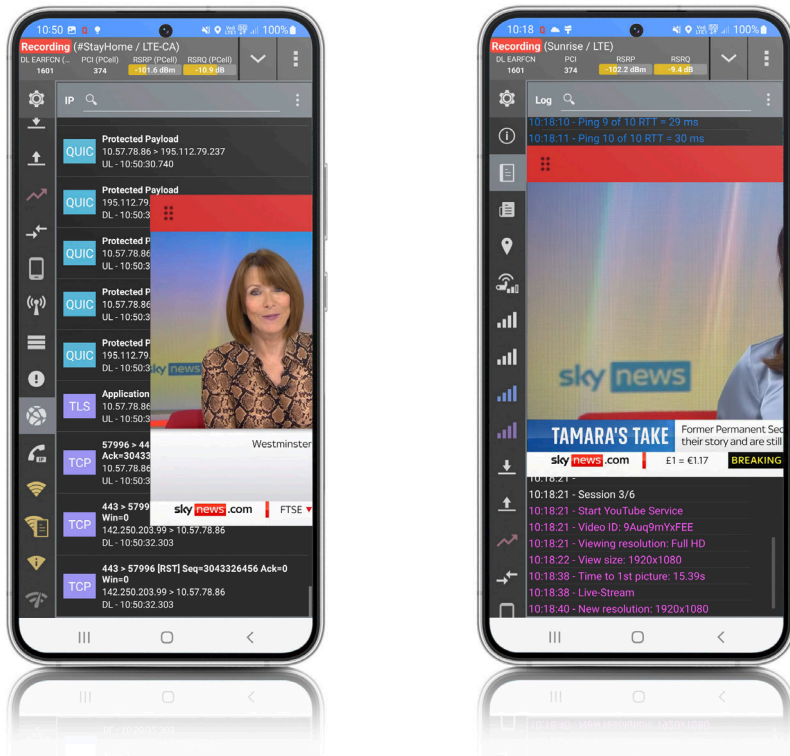
Fig. 8: Real-time analysis of a YouTube video with QualiPoc Android based on the flowchart in Fig. 7
