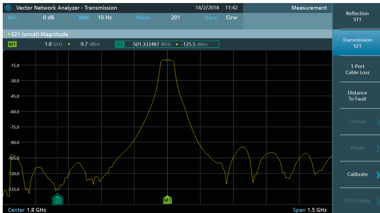
R&S®FPC1500 S_{21} scalar transmission measurement with the R&S®FPC-K42 option
