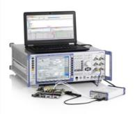
Combined with the R&S®RT-ZVC multichannel probe, precise measurements of current, voltage and power can be made while being tightly synchronized with network signaling events
