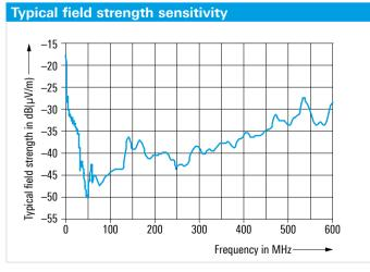
At antenna output (measurement bandwidth  $\Delta f = 1$  Hz; S/N = 0 dB).
