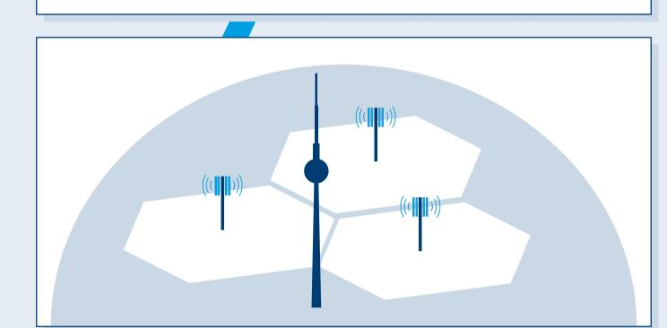
**SDL** (Supplementary Downlink): An additional frequency resource to increase the capabilities of base stations for the downlink only (from network to mobile devices) in order to enable much higher data rates for the downlink than for the uplink direction.
