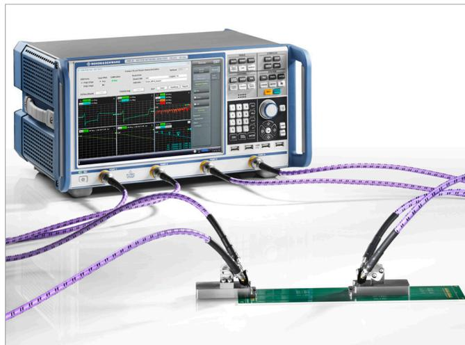
Besides the actual signal trace to be measured, PCB test coupons typically also include a shorter signal trace to facilitate this deembedding. Differential PCB probes (e.g. from PacketMicro) are used to connect the R&S®ZNB20 to these signal traces.
