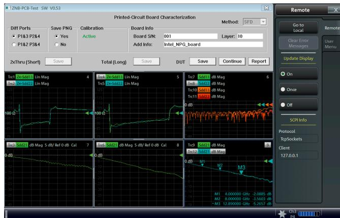
For the 2xthru (short) as well as for the total (long) measurement, the impedance versus time of both probes is displayed above the insertion loss. This makes it easy to quickly identify whether a probe needs to be readjusted.
