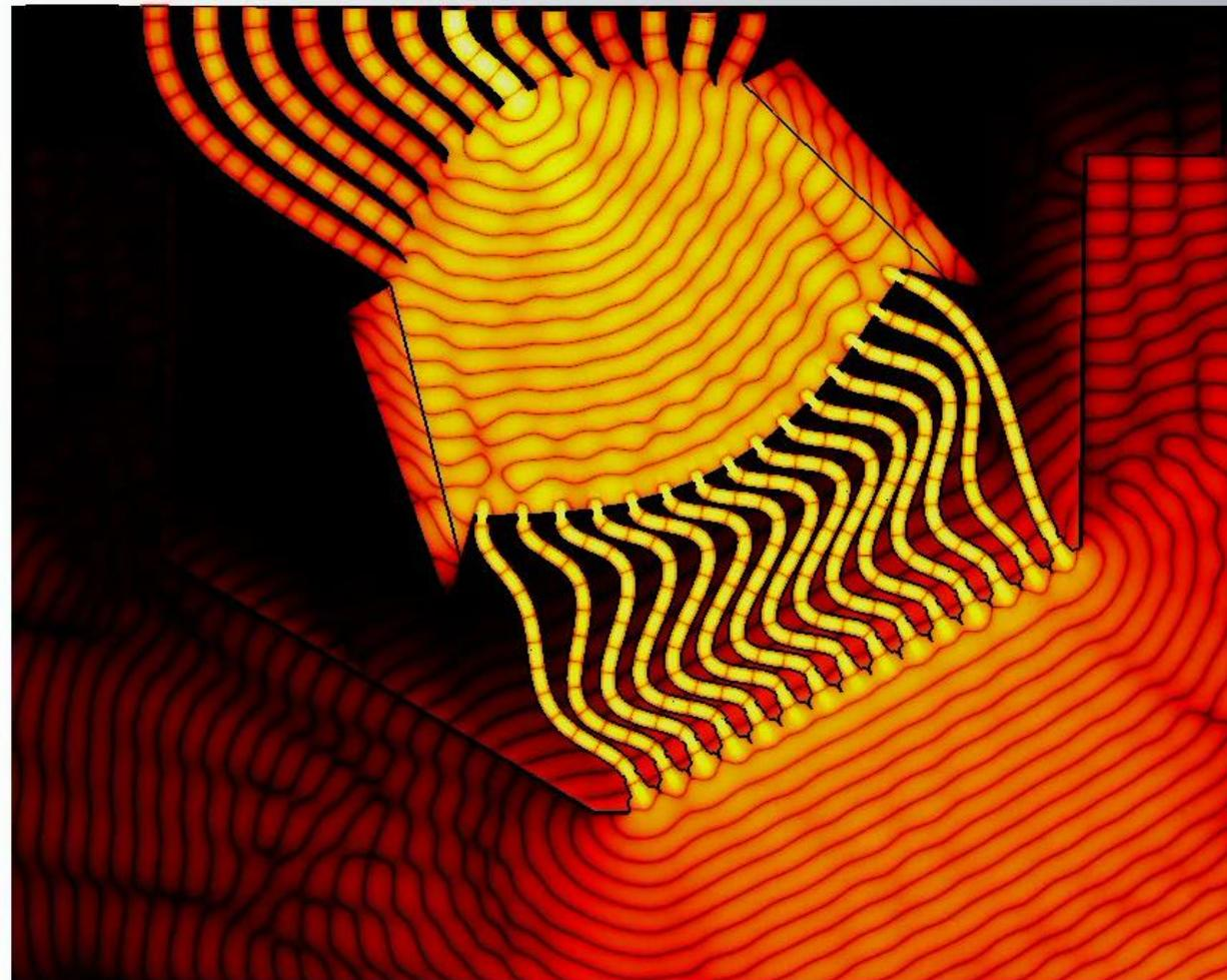
Electromagnetic lens for power distribution
