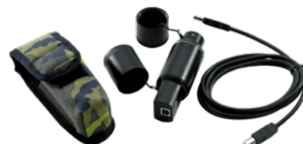
R&S®GP3021 fillgun For transmitting all relevant preset information as well as COMSEC/TRANSEC keys
