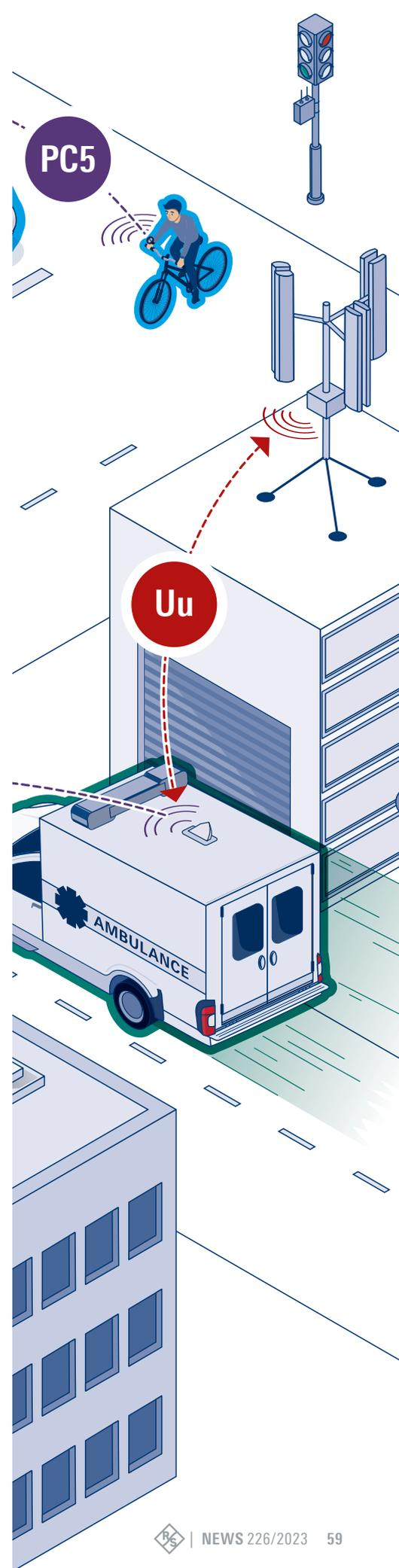
vehicle-to-everything (V2X) communications. It includes vehicle-to-vehicle (V2V), vehicle-to-infrastructure (V2I) and vehicle-to-pedestrian (V2P) communications.
