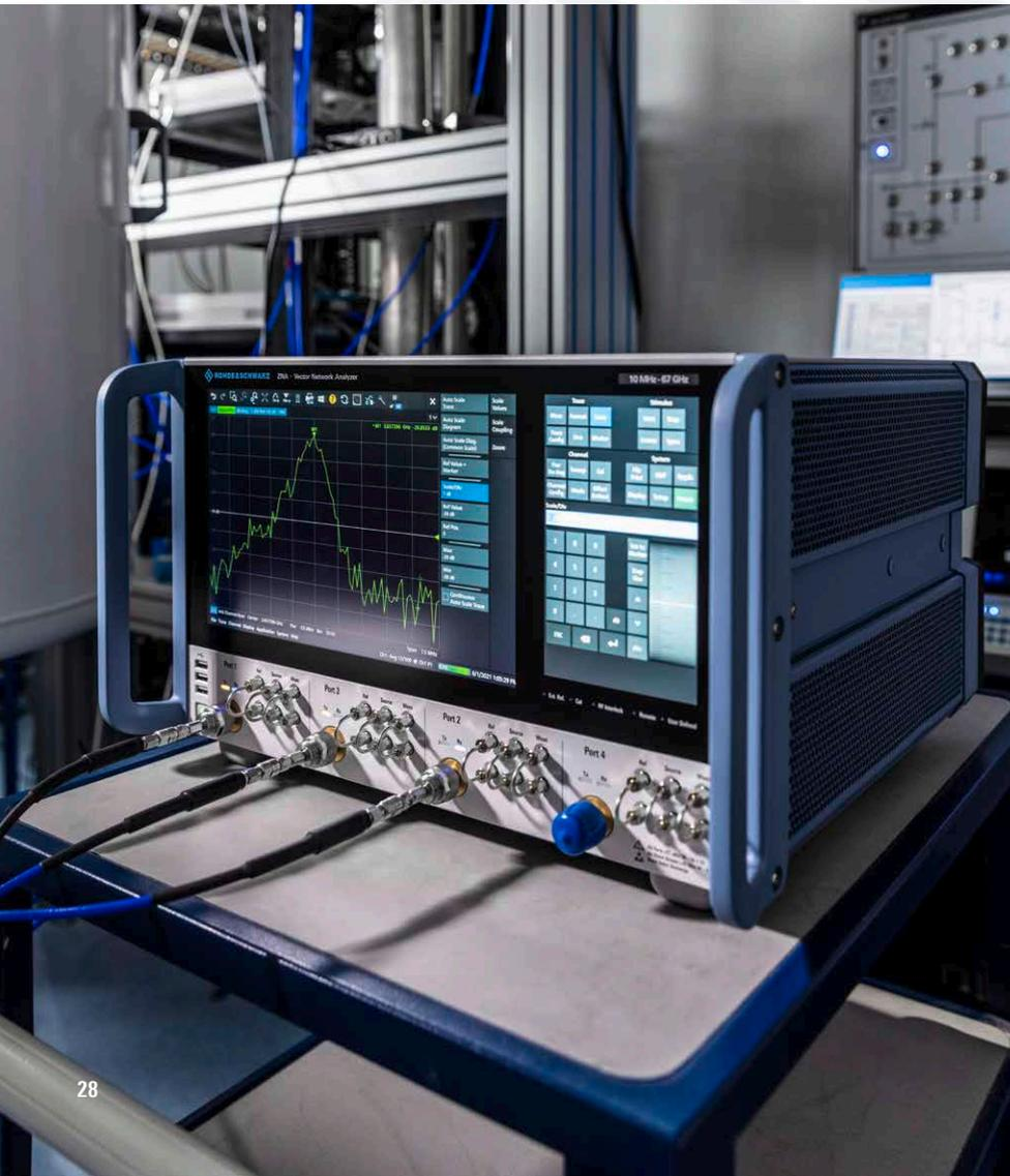
Fig. 3: Measurement setup at the Walther-Meißner-Institute with a cryostat (right) and an R&S®ZNA vector network analyzer (left) for analyzing the resonances of superconducting circuits.
