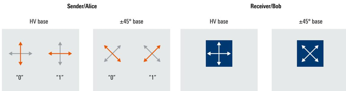
Fig. 2: In the horizontal-vertical base (HV), vertical polarization represents a bit value of zero and horizontal polarization a bit value of one. This applies analogously in the rotated 45° base.
