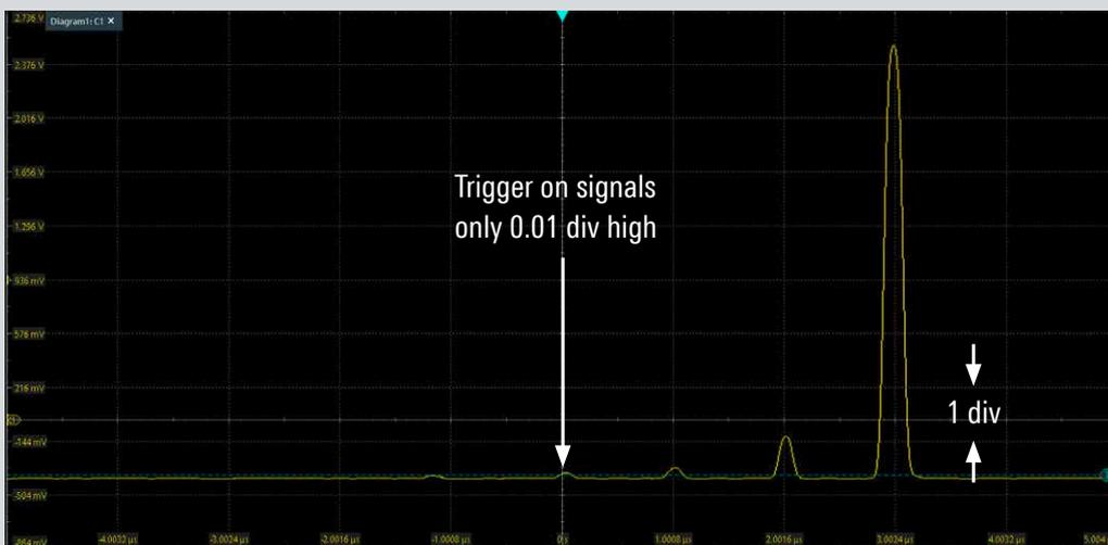
Fig. 2: The R&S®MXO 4 offers the industry's most sensitive trigger of 1/10000 vertical division and maintains a very short trigger rearm time of < 21 ns.
