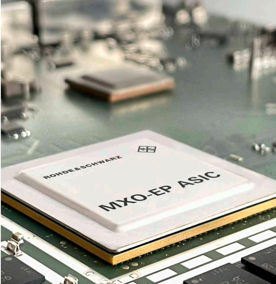
Fig. 3: A new 200 Gbit/s ASIC inside the R&S®MXO 4 was custom-developed for signal processing.
