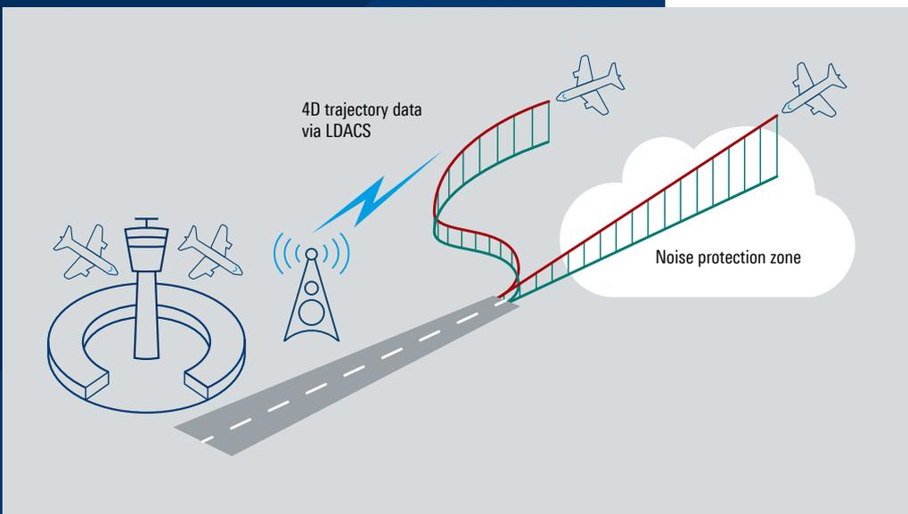
Fig. 1: Example of a 4D trajectory. When flying around noise protection zones in the future, more complicated maneuvers will be required instead of a straight approach. Pilots will obtain position data via the LDACS data link.
