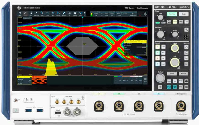
Eye diagrams give a quick overview of data signal jitter and noise while also revealing the robustness of data transmissions. Numerous fast bus interface standards, such as USB and PCI Express (PCIe), now define eye masks for signal integrity testing, clearly illustrating their importance.
