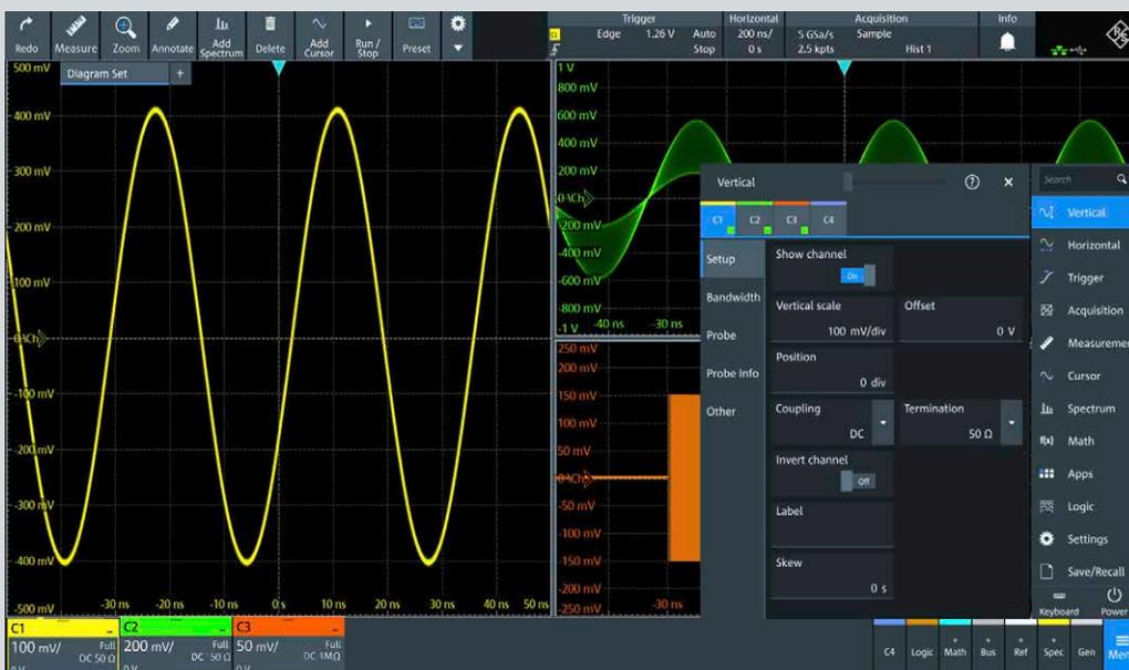
Fig. 5: Waveform viewing is maximized even when setting dialogs are open. This fulfills a key user requirement.
