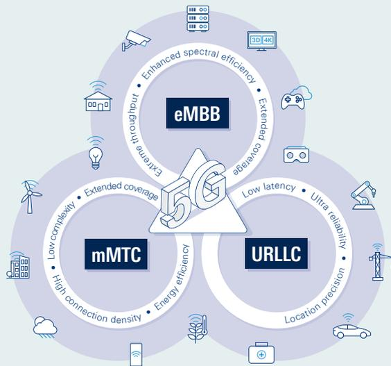
Fig. 1: 5G aims to cover three application groups. Enhanced mobile broadband (eMBB) allows classic mobile applications but with much better performance than LTE. Massive machine type communications (mMTC) supports energy efficient low-performance applications such as sensor networks. Ultra-reliable, low latency communications (URLLC) focuses on real-time applications that require ensured signal transit times and availability.
