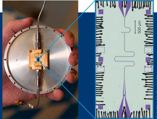
Fig. 4: Structure of a superconducting parametric amplifier.
