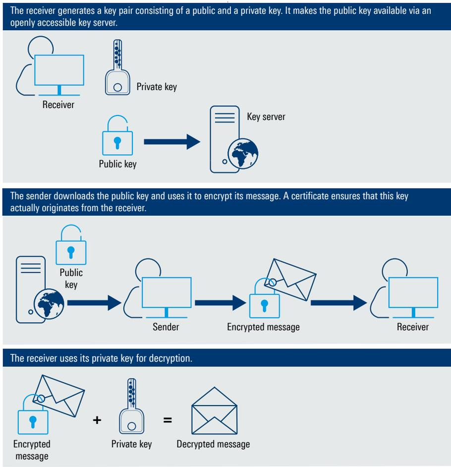
Fig. 1: Basic principle of asymmetric cryptography.
