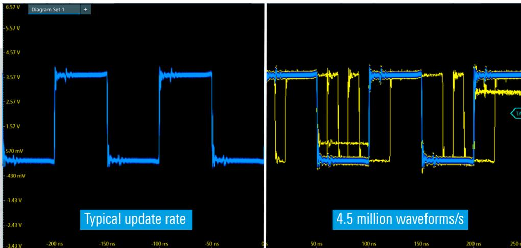
Fig. 1: An update rate of 4.5 million waveforms per second helps detect signals that could be missed otherwise.
