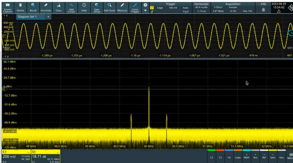
Fig. 4: The R&S®MXO 4 spectrum function offers the familiar interface of a spectrum analyzer.
