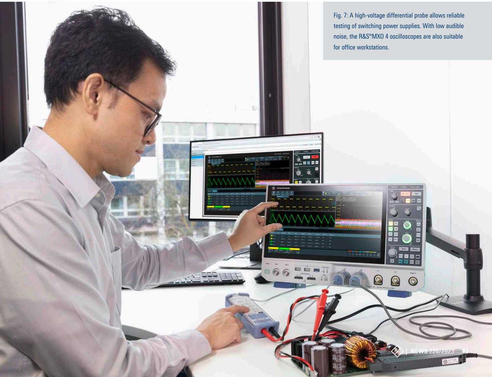
Fig. 7: A high-voltage differential probe allows reliable testing of switching power supplies. With low audible noise, the R&S®MXO 4 oscilloscopes are also suitable for office workstations.
