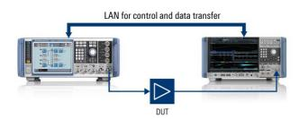
The measurement setup includes an R&S°FSW or R&S°FSV(A)3000 signal and spectrum analyzer or R&S°VSE compliant instruments with an R&S°SMW200A, R&S°SMM100A or R&S°SMBV100A vector signal generator. The closed-loop system enables control of the signal generator and automatic synchronization.
