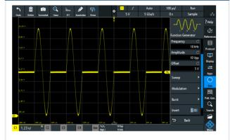
The R&S®RTx-B6 arbitrary waveform generator offers various user options, providing more flexibility for your applications. Besides different types of waveforms, the frequency, amplitude or offset can be set. For each waveform, you can configure the sweep and modulation type and add different burst signals.
